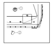
3. Tighten carburetor drain screw, and install carburetor drain cover.
